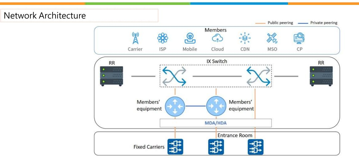
The network architecture of TWIX is composed of Ethernet Switches (E/S) and Route Reflectors (RR). The types of equipment are listed as follows. (1) E/S : Providing peering connection of FE/GE/10GE interfaces.
